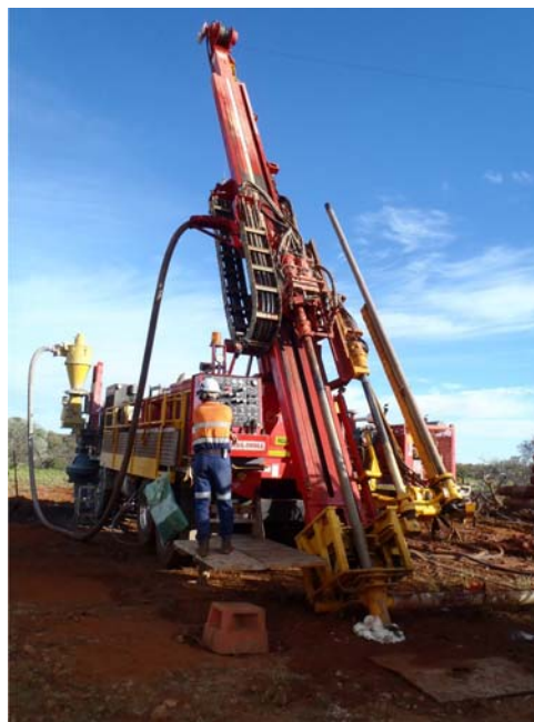
RC drilling using a Versadrill rig at Sabbath
